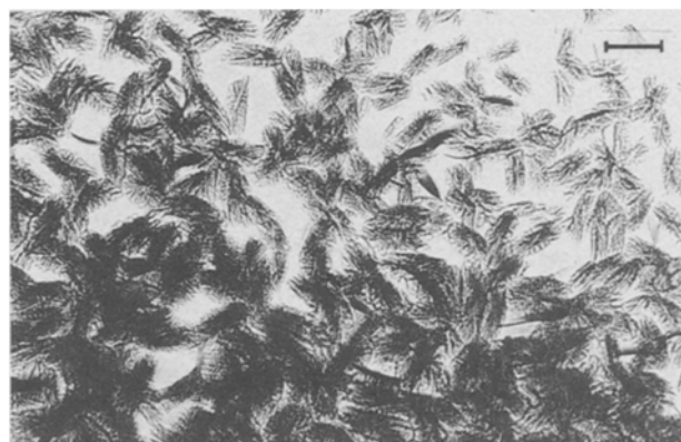
Figure 9 CPB1 glass heat-treated at 725^\circ\text{C} for 10 h. Optical transmission micrograph showing morphology of surface crystallization. Transmitted light normal to glass surface (bar denotes 50\ \mu\text{m} ).
